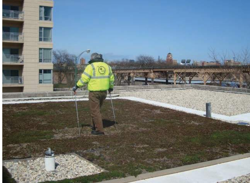
ELECTRONIC FIELD VECTOR MAPPING IN ACTION Images provided by: International Leak Detection
